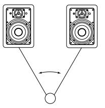
For best stereo imaging, we recommend that the units be placed so that the tweeters are as close as possible to the ear level of a seated listener. As this is not always possible in keeping with aesthetic design of a particular room, MTX In-Wall Speakers were designed with a pivoting tweeter which rotates to allow you to "aim" the high frequencies toward the listening position.
